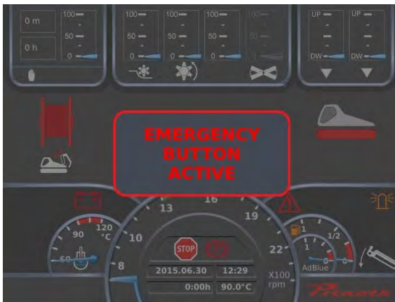
Figure 67: Emergency OFF switch active message
