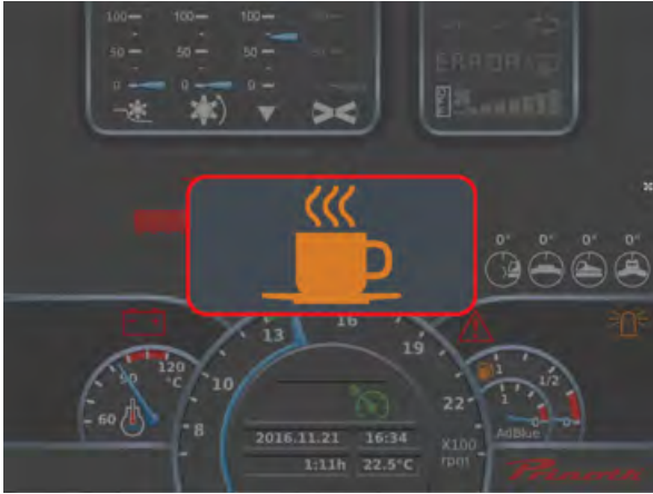
Figure 69: Icon and acoustic alarm triggered by lack of activity
