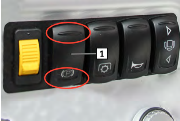
Figure 76: Rocker switches on the control console
